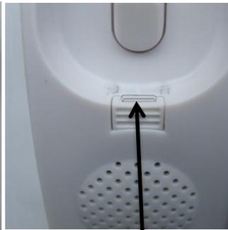
Insert Handset wall clip with tongue protruding (slide out and rotate as required)
